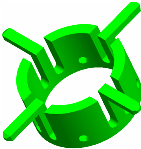
Fig. 4. Centering thimble design.
