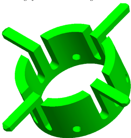
Axisymmetric model of a centering thimble
